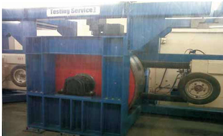
Endurance Testing Machine
