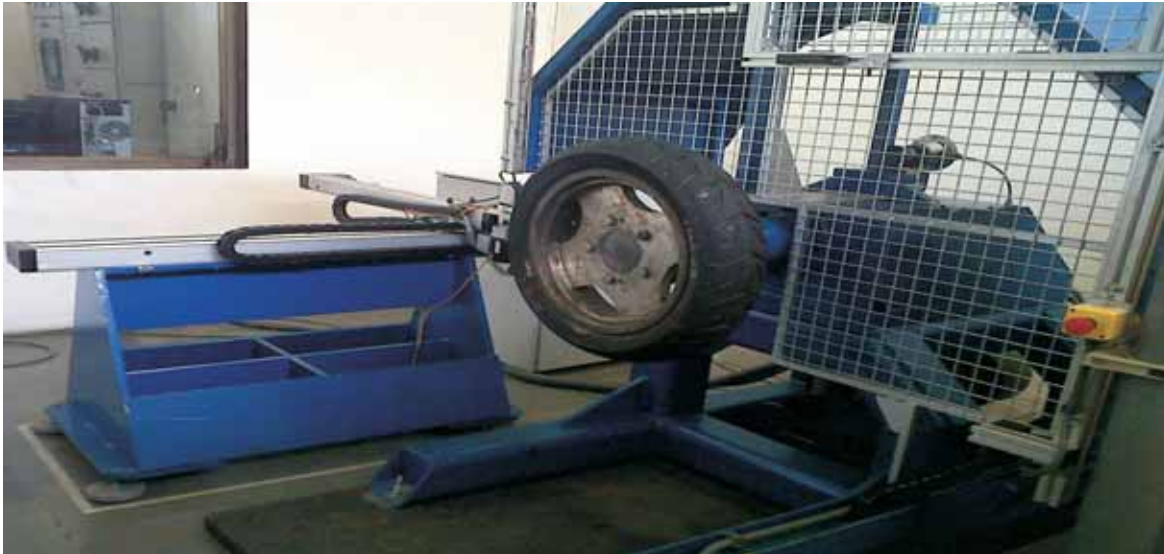
Dynamic Growth (Tyre Profilometer) Machine
