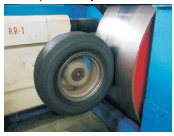
Our tyre testing centre has developed the required expertise for testing the rolling resistance of tyres as per international standards and made very good comparison with internationally reputed tyre testing centres. Our facility is being extensively used by many automotive OEMS for testing the rolling resistance tyres for their new models and also for bench marking the quality of tyres from different manufacturers
