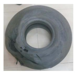
Most of the failed fighter aircraft tyres so far investigated found to have failure due to localized excessive wear and degradation resulting in tyre burst. The shearography has also been used for the investigation of unused aircraft tyres having surface defects.
